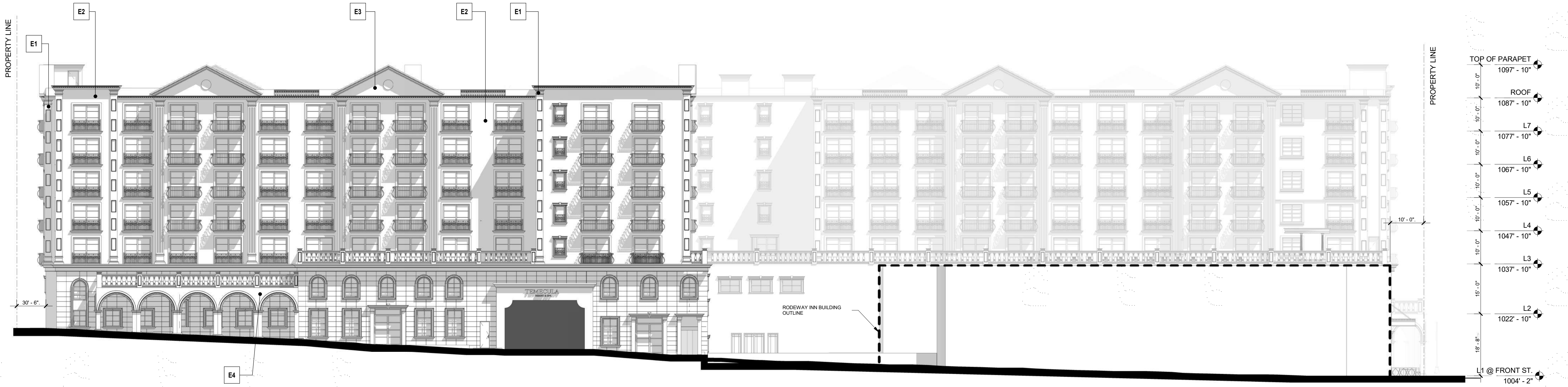
A BUILDING ELEVATION @2ND STREET SCALE 1/16" = 1'-0"
