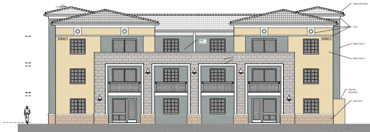
Buildings #11 (Type H) Long Side Elevation Color Scheme 4 3/32" = 1'-0"
