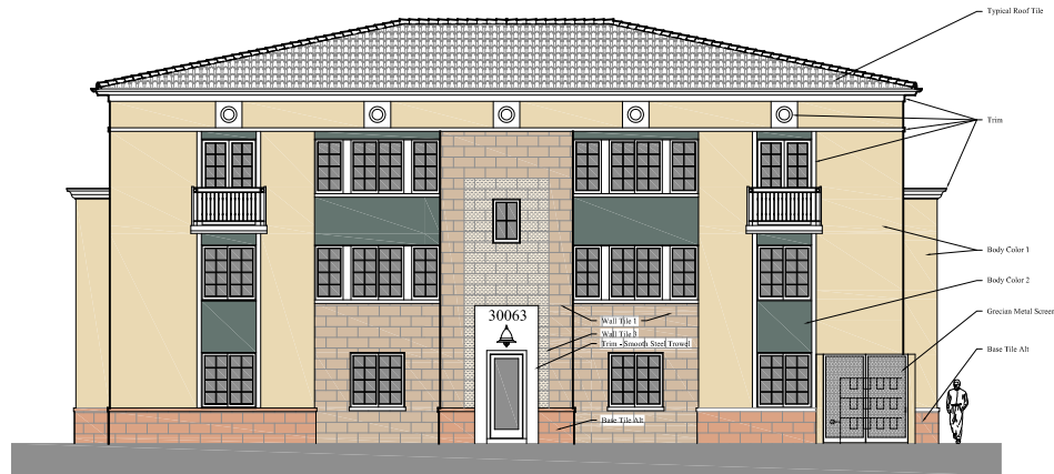
Building #12 (Type G) End Elevation Color Scheme 2 3/16" = 1'-0"
